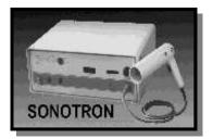
applied periodic bursts of radio-frequency energy whose repetition rate is at a sonic frequency and whose peak amplitude is such as to cause a corona discharge. This energy is derived from a radio-frequency carrier generator whose operating frequency is at 430 Khz. This carrier is over modulated in amplitude at a sonic rate, whose frequency is in the 1 - 5 Khz range, so that the carrier is interrupted periodically to produce the bursts.
